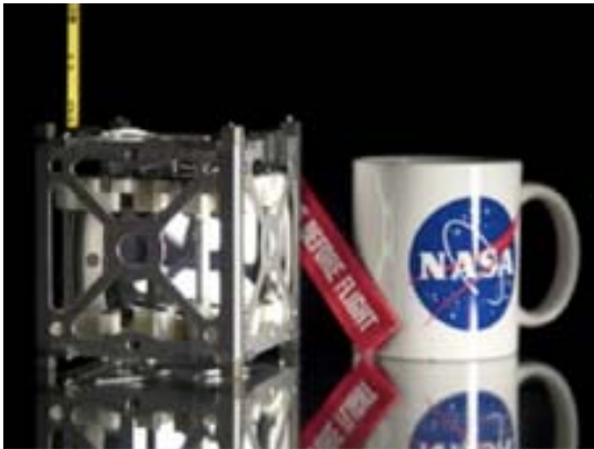
Figure 1: NASA's PhoneSat Nano-satellite, shown next to a coffee mug for size comparison.
